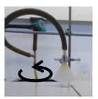
Put the glass petri dish below an upside-down funnel, connected to a venturi vacuum.
